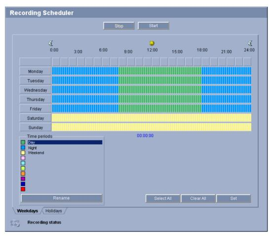
The recording scheduler allows you to link the created recording profiles with the days and times at which the camera's images are to be recorded in the event of an alarm. You can link any number of 15-minute intervals with the recording profiles for each day of the week. Moving the mouse cursor over the table displays the time below it. This aids
